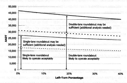
This is a planning level capacity analysis diagram. Up to about 18,000 AADT, depending on left turn percentages, a single lane roundabout is likely to operate. At more than 18,000 AADT, a single lane roundabout may be sufficient.
